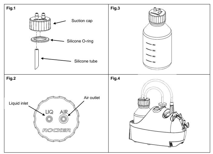
See Fig.2: Connect "LIQ" (Liquid inlet) to suction kit and connect "AIR" (air outlet) to vacuum source.
