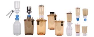
Lafil series vacuum filtration system can be used with a variety of filtration ware for different applications.
