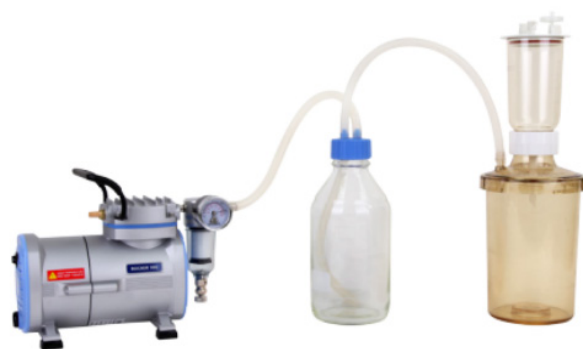
Using a safety bottle to prevent from overflowing
